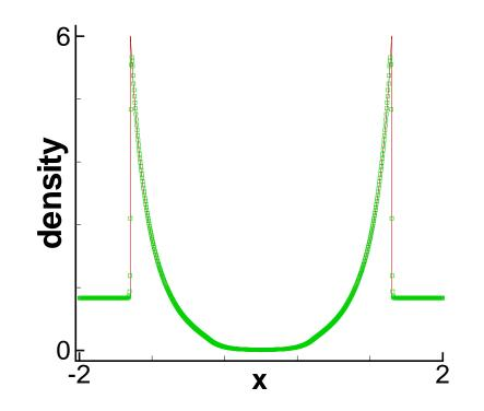
Figure 4: 1D Sedov blast. The solid line is the exact solution. Symbols are numerical solutions. T = 0.001. N = 800.  $\Delta x = \frac{4}{N}$ . TVB limiter parameters  $(M_1, M_2, M_3) = (15000, 20000, 15000)$ . Density.
