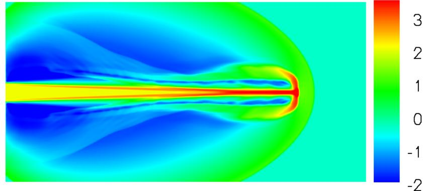
Figure 13: Simulation of Mach 80 jet without radiative cooling. Scales are logarithmic. Density.
