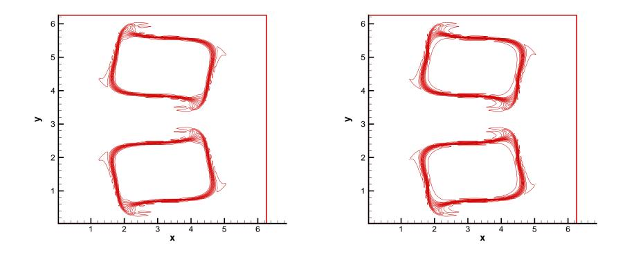
Figure 1: Vorticity at t = 10,  $P^2$ . 30 equally spaced contours from -1.1 to 1.1.  $128^2$  mesh. Left: with limiter; Right: without limiter.
