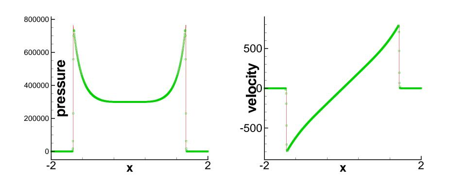
Figure 3: 1D Sedov blast. The solid line is the exact solution. Symbols are numerical solutions. T = 0.001. N = 800.  $\Delta x = \frac{4}{N}$ . TVB limiter parameters  $(M_1, M_2, M_3) = (15000, 20000, 15000)$ . Pressure (left) and velocity (right).
