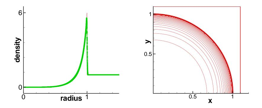
Figure 5: 2D Sedov blast, plot of density. T = 1. N = 160.  $\Delta x = \Delta y = \frac{1.1}{N}$ . TVB limiter parameters  $(M_1, M_2, M_3, M_4) = (8000, 16000, 16000, 8000)$ .
