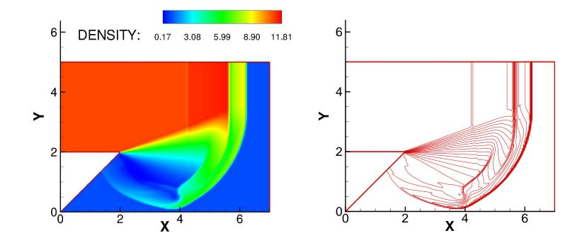
Figure 16: Density. Detonation diffraction at a  $135^{\circ}$  corner.
