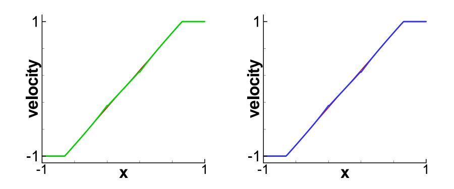
Figure 9: Double rarefaction problem. T=0.6. Left: 1D problem. Right: Cut at y = 0 for the 2D problem. Every fourth cell is plotted. The solid line is the exact solution. Symbols are numerical solutions.  $\Delta x = \frac{2}{N}$ , N = 800 with the positivity limiter. Velocity.
