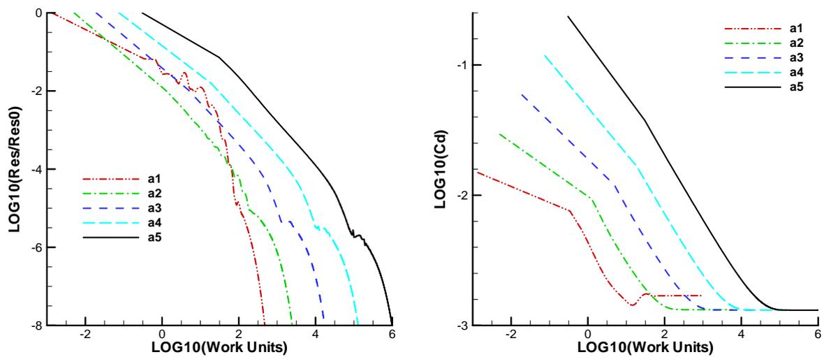
Fig. 1 Convergence histories for the computation with different meshes
