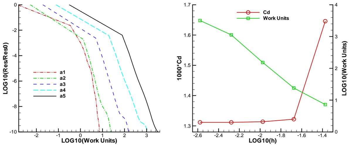
Fig. 4 Convergence histories, drag coefficients and computational costs for grid refinement with implicit method
