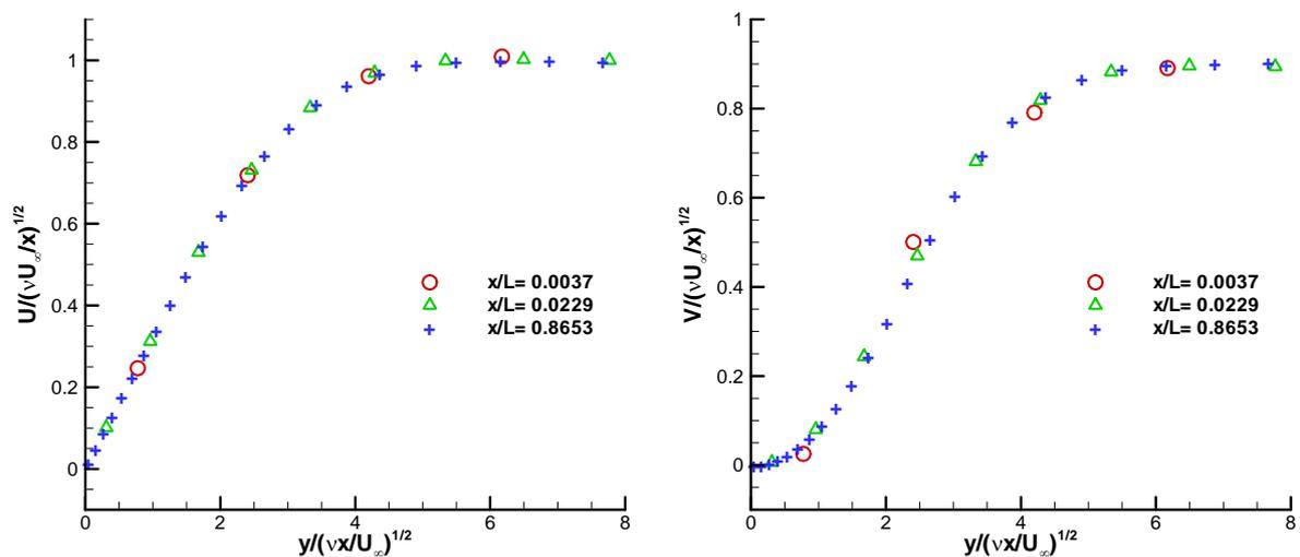
Fig. 2 Streamwise and transverse velocity profiles at different streamwise locations (a3 mesh)
