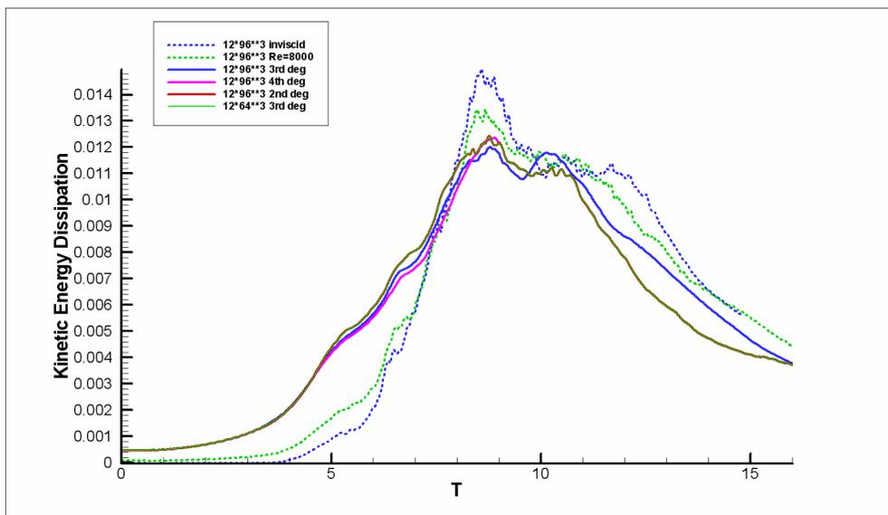
Figure 4 : Scaled kinetic energy dissipation for the C3.5 case and lower viscosity cases
