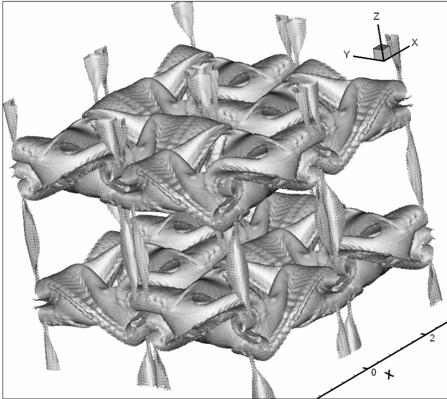
*Figure 10 : Isosurface Enstrophy = 1. before the transition in the run at Reynolds = 8000*
