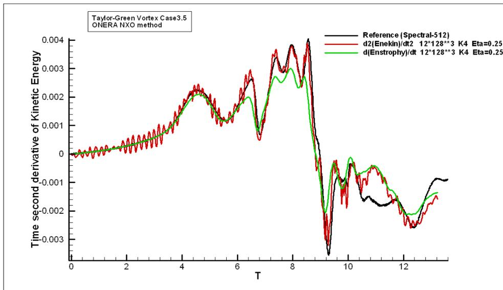
Figure 6 : Time derivatives of the volume integrals of enstrophy and scaled dissipation
