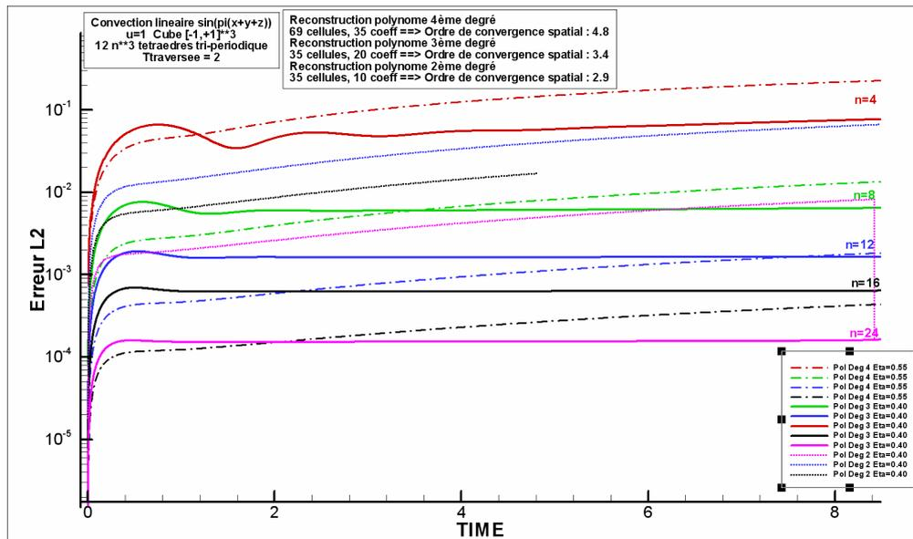
Figure 1 : Norm of the error in time for the convection of the function  $\sin(x+y+z)$  in a 3-periodic cube meshed by tetrahedra
