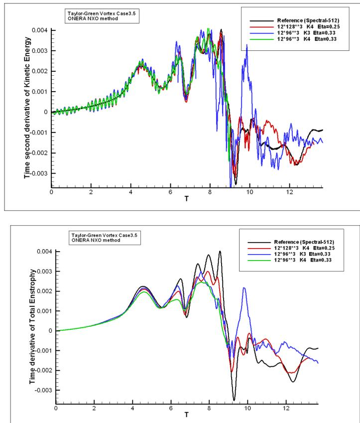
Figures 7 and 8 : Time derivatives of the scaled integral dissipation and of the volume integral of enstrophy
