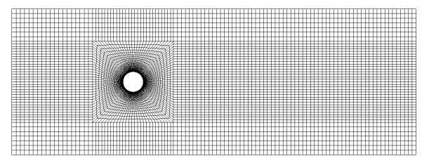
Fig. 3. Coarse mesh in X-Y plane
