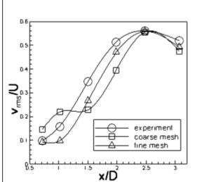
Fig. 16(a). Distribution of the streamwise r.m.s. velocities along the wake centerline.
