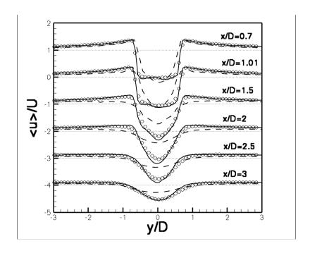
Fig. 9. Mean normalized streamwise velocity in the wake of the circular cylinder, (0000) - experiment; (Dashed line) –  $2^{nd}$  order results; (Solid line) –  $3^{rd}$  order results. The dotted line (.....) represents the zero location of the shifted curves.
