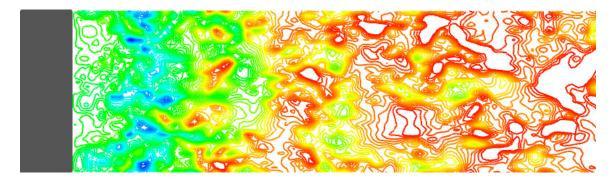
Fig. 5. Instantaneous streamwise velocity in x-z plane (y=0) in the wake of the cylinder. There are 40 contours from -0.1 to 0.1.
