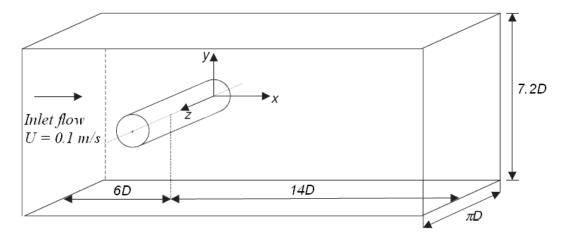
Fig. 2. The geometry of the flow over cylinder
