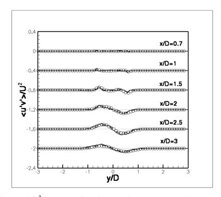
Fig. 15. Normalized <u'v'>/U $^2$  in the wake of the circular cylinder, (0000) - experiment; (Dashed line) - coarse mesh; (Solid line) - fine mesh. The dotted line (.....) represents the zero location of the shifted curves.
