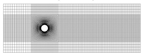
Fig. 4. Fine mesh in X-Y plane
