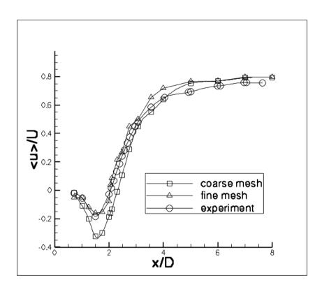
Fig. 12. Distribution of the streamwise mean velocity along the wake center-line.
