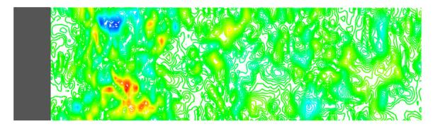
Fig. 7. Instantaneous spanwise velocity in x-z plane (y=0) in the wake of the cylinder. There are 52 contours from -0.1 to 0.1.
