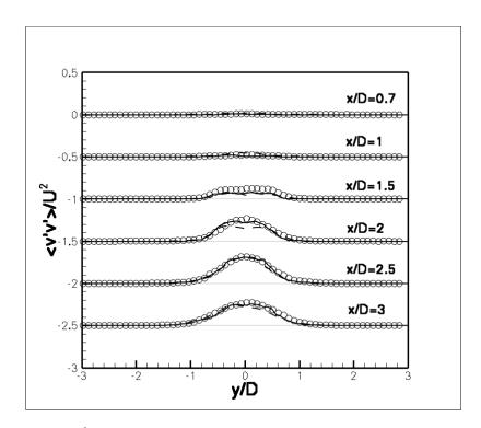
Fig. 14. Normalized  $\langle v'v' \rangle / U^2$  in the wake of the circular cylinder, (0000) - experiment; (Dashed line) – coarse mesh; (Solid line) – fine mesh. The dotted line (.....) represents the zero location of the shifted curves.
