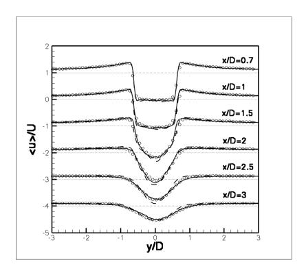
Fig. 10. Mean normalized streamwise velocity in the wake of the circular cylinder, (0000) - experiment; (Dashed line) - coarse mesh; (Solid line) - fine mesh. The dotted line (.....) represents the zero location of the shifted curves.
