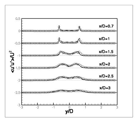
Fig. 13. Normalized <u'u'>/U $^2$  in the wake of the circular cylinder, (0000) - experiment; (Dashed line) – coarse mesh; (Solid line) – fine mesh. The dotted line (.....) represents the zero location of the shifted curves.
