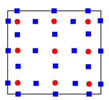
Fig. 1. Distribution of solution points (circles) and flux points (squares) in a standard element for a 3<sup>rd</sup> order SD scheme.
