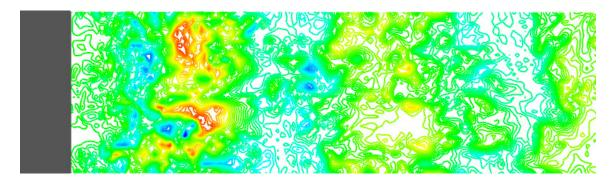
Fig. 6. Instantaneous transverse velocity in x-z plane (y=0) in the wake of the cylinder. There are 40 contours from -0.1 to 0.1.
