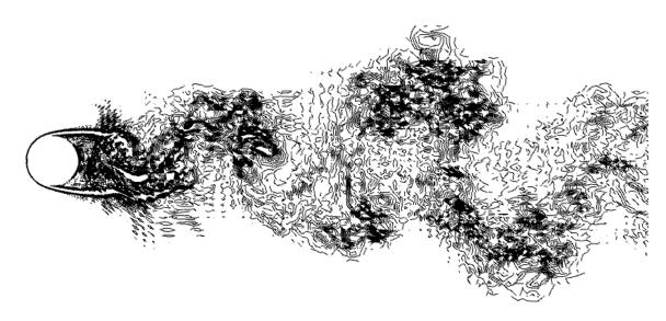
Fig. 8. Instantaneous vorticity magnitude showing 16 contours from  $\omega D/U = -0.1$  to  $\omega D/U = 0.1$ .
