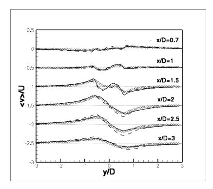
Fig. 11. Mean normalized transverse velocity in the wake of the circular cylinder, (0000) - experiment; (Dashed line) - coarse mesh; (Solid line) - fine mesh. The dotted line (.....) represents the zero location of the shifted curves.
