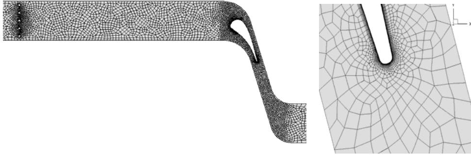
Figure 22. FR/CPR unstructured computational mesh for the uncooled VKI S1N.
