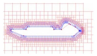
Figure 2(b). Formation of Interpolation-Based Hybrid Grids: The Interpolation-Based Treatment Retains a Sufficiently Thick Overlap Layer Between the Cartesian and Prism Cells for Use in Solution Interpolation
