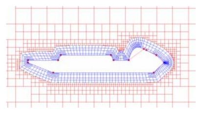
Figure 2(a). Formation of Conservative Hybrid Grids: The Conservative Treatment is Based on Cutting the Cartesian Cells and Eliminating All Overlapped Cartesian Cells and Cell Fragments From the Hybrid Grid
