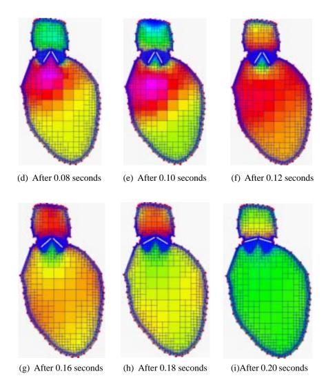
Figure 4. Grid, Geometries, and Pressure Distributions at Various Times During a Complete Cycle of an Artificial Valve Fitted to a Human Heart (*cont.*)
